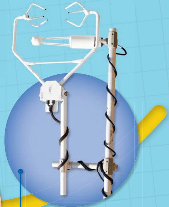
An ultrasound anemometer has pairs of sound speakers and microphones. Electronic circuits measure the time it takes for sound to travel from each speaker to its microphone. The anemometer uses the data collected to determine wind speed as well as wind direction.
