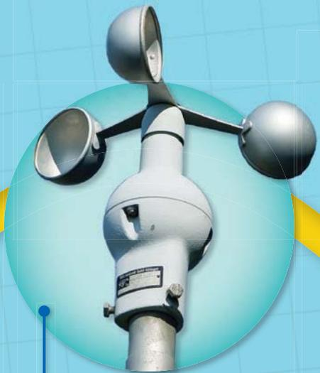
This anemometer uses cuplike devices to measure wind speed. The faster the wind blows, the faster the cups spin. The cups are attached to sensors that measure the actual wind speed.
