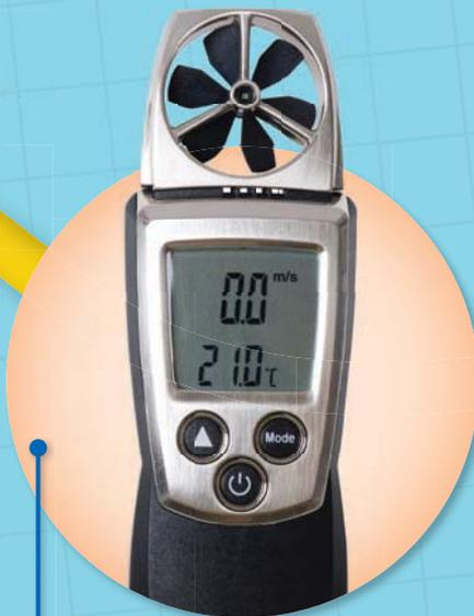
This digital anemometer uses spinning fans to generate magnetic pulses. Then the instrument translates these pulses into measurements of the wind speed.
